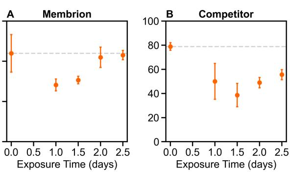
Figure 4. Performance of Membrion and competitor resins after exposure of 35%  $H_2O_2$ . Adsorbed moles of AO7 per unit resin mass with respect to hydrogen peroxide exposure time for (**A**) Membrion and (**B**) competitor resins. Points and bars represent mean ± 1 standard deviation (n = 3).
