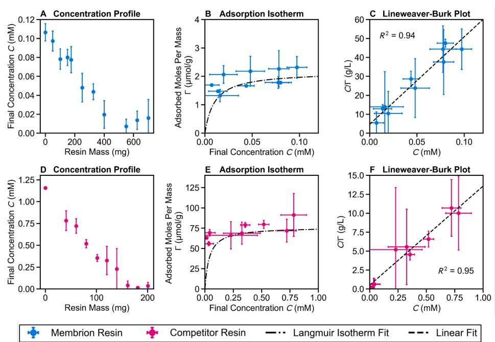
Competitor resin can treat more concentrated AO7 solution with less resin mass Competitor resin (76 µmol/g) has one order of magnitude higher moles of AO7 adsorbed in a closed packed monolayer compared with Membrion resin (2.2 µmol/g) Linear Lineweaver-Burk plot suggests both resins are described by Langmuir isotherm
